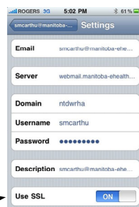
[9] Return to the Settings for your newly created account and ensure that Use SSL is turned ON
